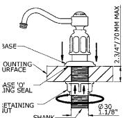
The diameter of the hole should be Ø30mm/1.1/8". The maximum thickness of the surface must not exceed 70mm/2.3/4"
